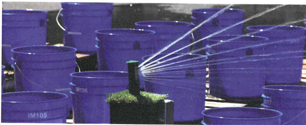
Figure 4 – Digital Sprinkler Test, Northern Water
