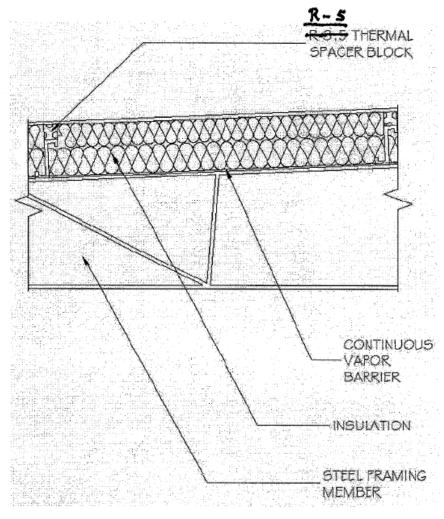
SECTION VIEW OF METAL FRAME ROOF:
