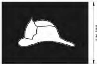
FIGURE 3007.6.5 FIRE SERVICE ACCESS ELEVATOR SYMBOL
